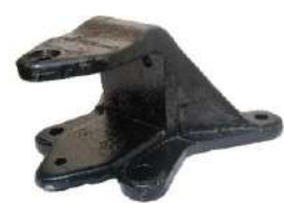
Item Code: AKAL3842 REAR SPRING REAR BRACKET M12 PIN BHARAT BENZ 3723 OEM NO.A4003 250 003 MRP: Rs.3780
