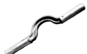
Item Code: AKAL5285 TRUNION SHAFT NEW MODEL LEYLAND U-TRUCK O.D. MRP: Rs.43260
