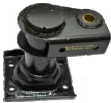
Item Code: AKAL1131 R/S REAR HANGER W/BUSH RH N/M TATA 407 N/M OEM NO.2651 3240 0136 MRP: Rs.2342
