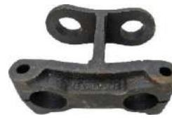
Item Code: AKAL3804D FRONT SPRG REAR SHACKLE 'H' TYPE BHARAT BENZ 1214R OEM NO.5A241FLM2 MRP: Rs.1885
